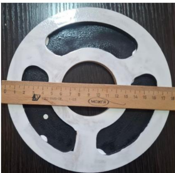
Figure 2 – Schematic drawing of the experimental saw spacers planned to be manufactured to improve the saw cylinder of the 5LP linter
