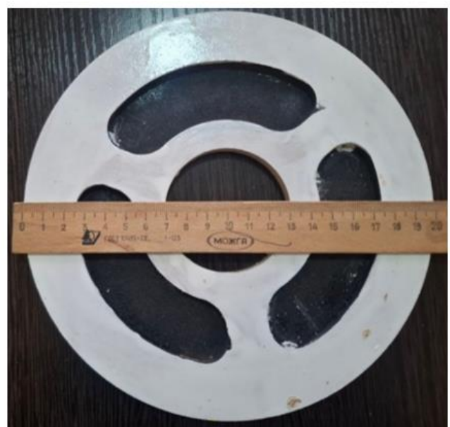
Figure 2 – Schematic drawing of the experimental saw spacers planned to be manufactured to improve the saw cylinder of the 5LP linter
